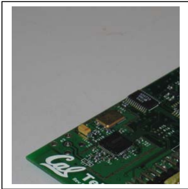
Figure 1 Wireless node carrying a sensor board at lower right with the MEMS accelerometer
